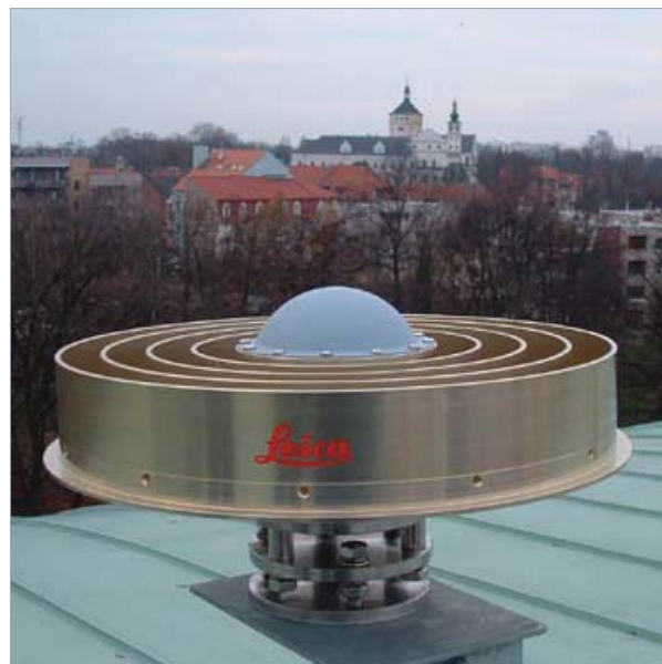
GPS stanice CZEPOS - Pardubice. CZEPOS GPS station - Pardubice.
